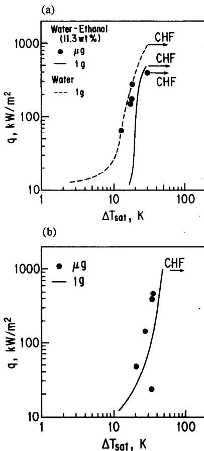
FIG. 10. Comparison of boiling curves under microgravity and 1g. (a) 11.3 wt% ethanol, (b) 27.3 wt% ethanol.
