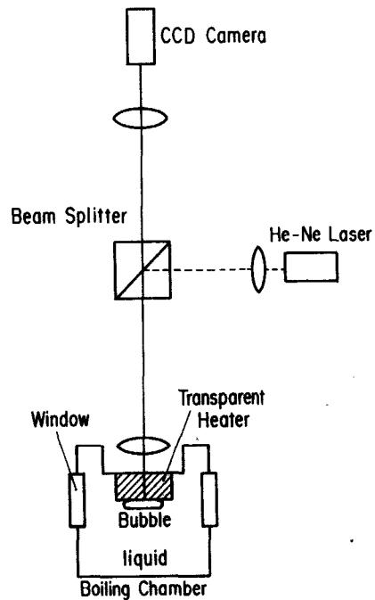
FIG. 7. Experimental set-up for interferometric observations.
