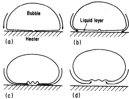
FIG. 5. Schematic illustration of bubble detachment mechanism.
