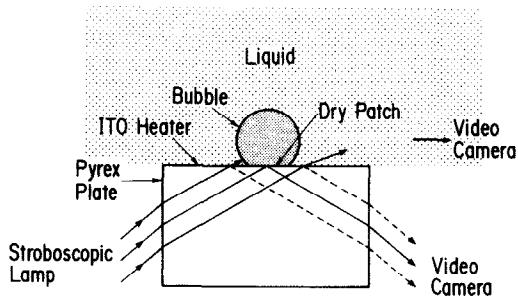
FIG. 1. Principle of observation with a transparent glass heater.
