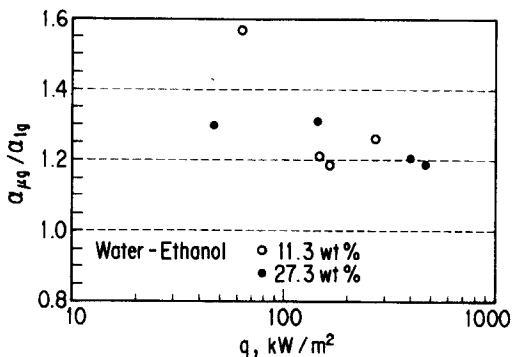
FIG. 11. Ratio of boiling heat transfer coefficient under microgravity to that under 1g.
