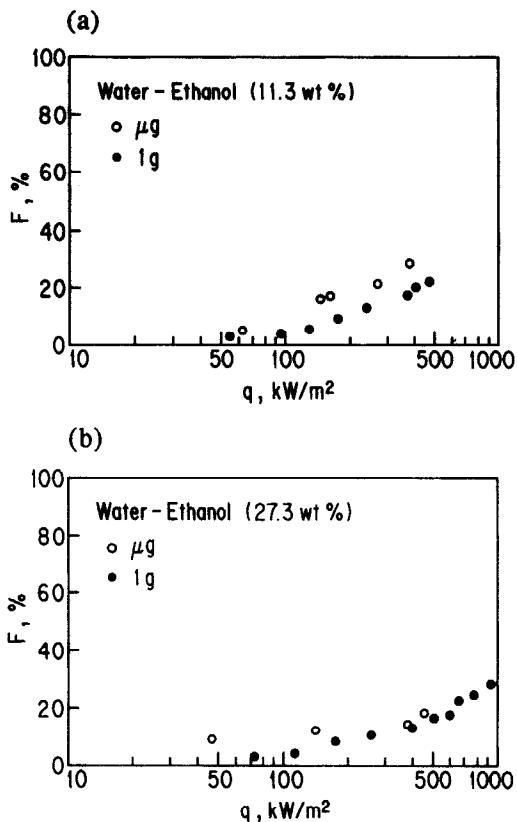
FIG. 9. Fraction of bubble/heater contact area plotted against heat flux. (a) 11.3 wt% ethanol, (b) 27.3 wt% ethanol.
